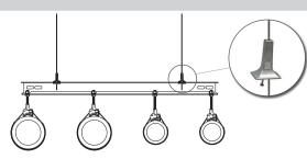
Suspended from the soffit using threaded rod or Trapeze No.2
